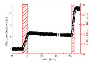
FIG. 1. (Color online) Photoconductance (black circles) of the  $VO_2$  device at 300 K, showing rapid increase during x-ray illumination (dashed red region) as well as slow decrease after the x-ray illumination was turned off.
